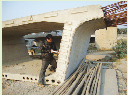
Rebound hammer test on a segment at Dabri Flyover, Delhi
