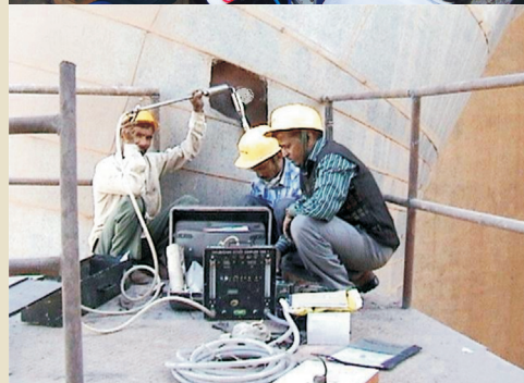
Monitoring of Gaseous Pollutants at Kiln Stack
