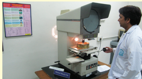
Calibration of sieve at Profile Projector
