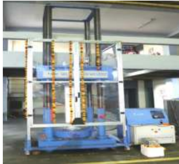
Column testing machine for checking behaviour of reinforced column
