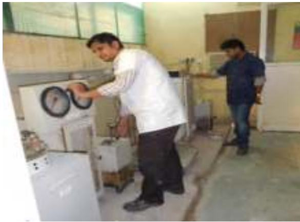
Testing Facility of Compressive Strength of Concrete Cube and Cement Mortar Cube
