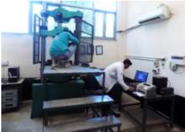
Universal testing machine- 1000kN for testing of reinforcement steel
