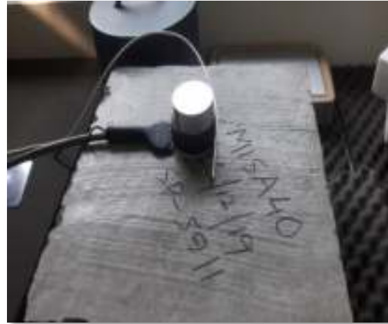
Determination of thermal conductivity and specific heat of concrete using TPS method
