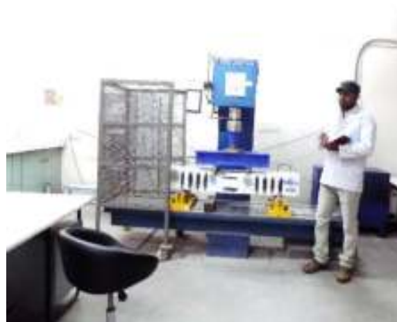
Flexural testing machine- 500kN for testing reinforced beam
