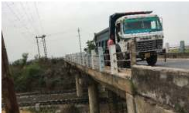
Determination of load carrying capacity by Load Testing of railway over bridge as per IRC SP-37 in progress at a sponsored project site
