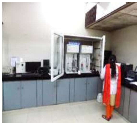
Mercury Intrusion Porosity equipment for checking porosity of concrete
