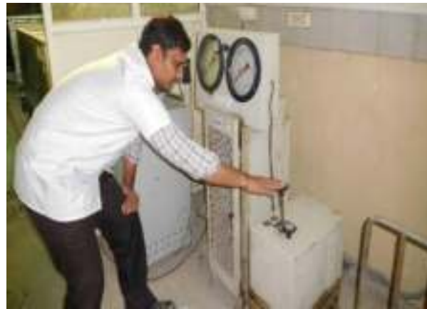
Testing Facility of Compressive Strength of Concrete Cube and Cement Mortar Cube
