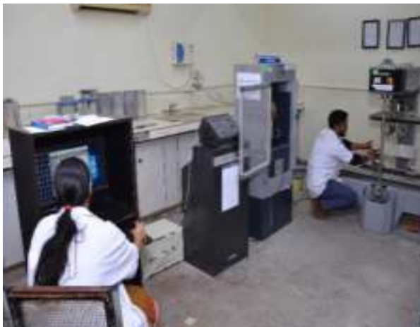
Strain Controlled Flexural Testing Machine for determination of flexural toughness of concrete
