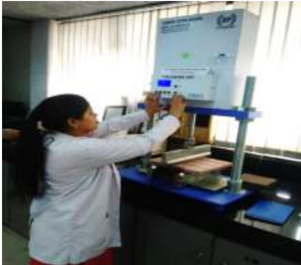
Flexural testing of cement concrete tile
