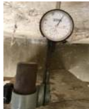
Determination of load carrying capacity by Load Testing of railway over bridge as per IRC SP-37 in progress at a sponsored project site
