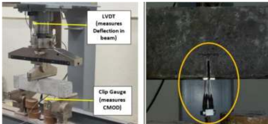
Experimental setup for evaluation of fracture parameters
