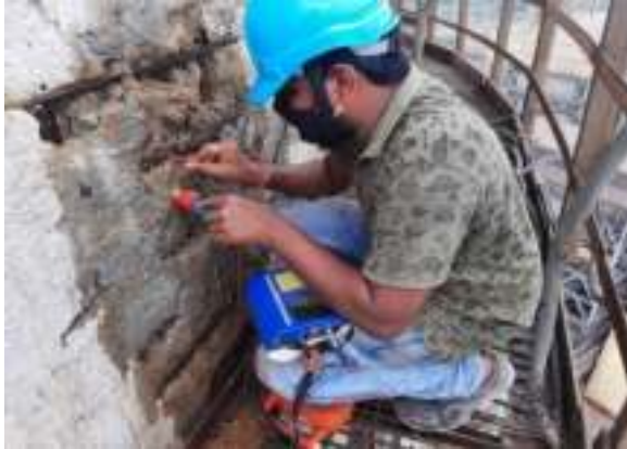
Non-Destructive Testing being carried out on RCC Chimney of NALCO, Angul, Odisha
