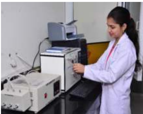
BET Apparatus for determining fineness of ultra- fine powder materials
