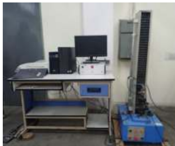
Steel fiber testing
