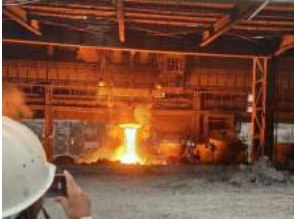
Visit of NCB team at Basic Oxygen Furnace (at plant of JSW Steel Limited at Bellary, Vidyanagar) where molten iron is converted to steel and BOF Slag or LD Slag is generated as by-product.
