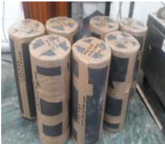
Butyl sheet wrapping to prevent moisture loss from specimen
