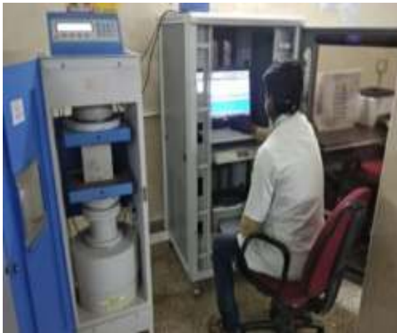
Water Permeability and Concrete Cube Testing being carried out at CDR Laboratory
