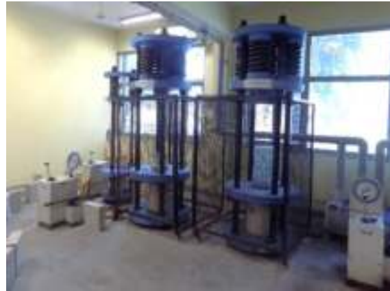
Creep Testing Machine for creep behaviour of concrete
