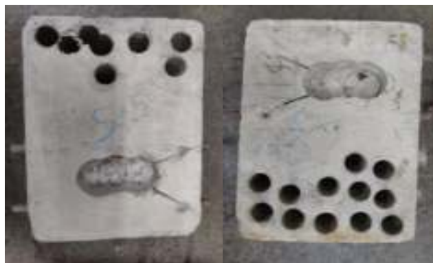
Preparation of specimens for installation of anodes
