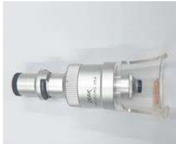
Portable Crack Width Observer
