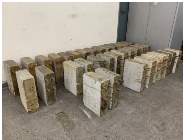
Samples cast for laboratory study under R&D project on Cathodic Protection of Reinforced Concrete
