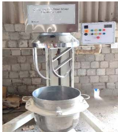
Planetary mixer developed at NCB for preparation of UHPC
