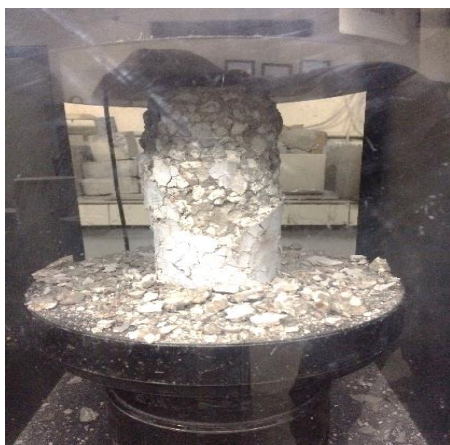
(a) Sample under testing after fire exposure
