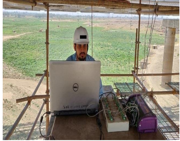
Strain measurement test on RCC girders for 400m PSC Bridge
