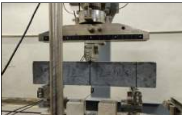
Test Setup for Three-point Bending of Beam Specimen for Fracture Study
