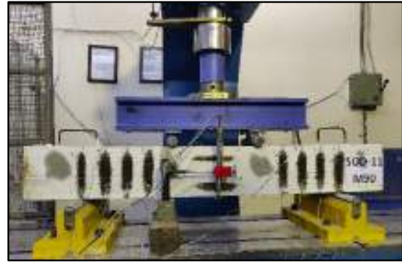
Testing of High Strength Concrete Reinforced Beams under progress in presence the of Dr B N Mohapatra, DG NCB, Sh V V Arora, Joint Director & Head-CDR & NCB Scientists
