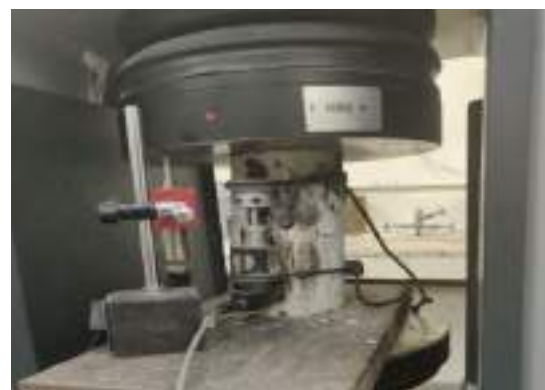
Test Setup for Modulus of Elasticity of Concrete Cylinder Exposed at 600° C
