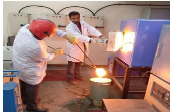
Fig. 8: Synthetic slag being produced in NCB Laboratory
