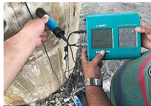
Half-cell Measurement test on Bridge Pier at NTPC Rihand
