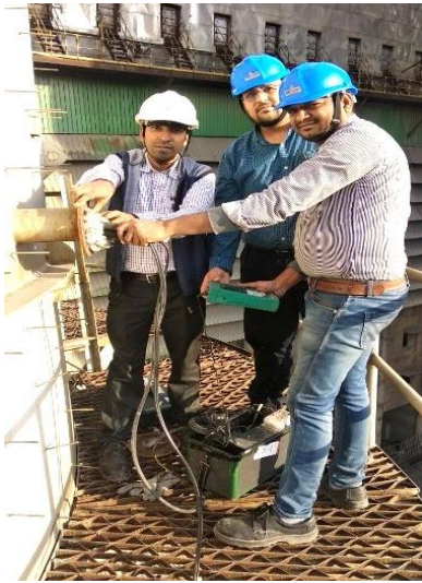
Measurements of SO 2 emissions at stack of a cement plant
