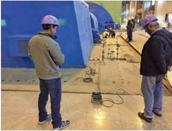
UPV Testing by Surface Probing on TG Deck Slab at APCPL, Jharli
