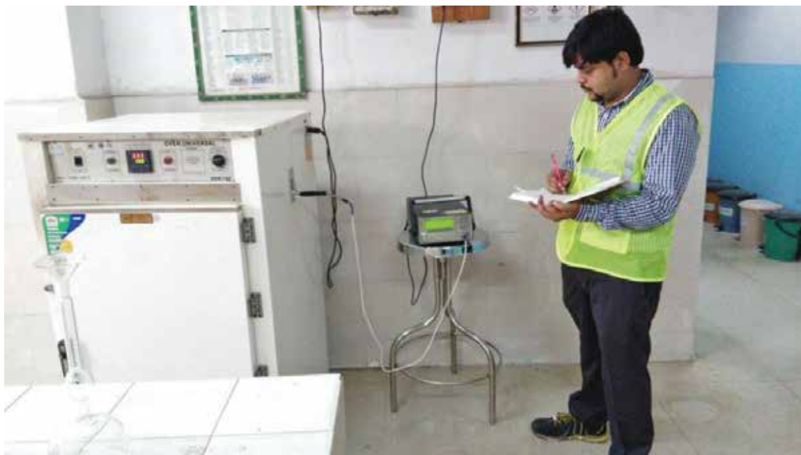
Calibration of Hot Air Oven in QC Laboratory of a Cement Plant
