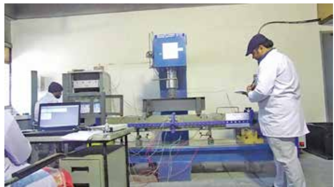
Test setup for Flexural Strength of Reinforced Concrete Beams
