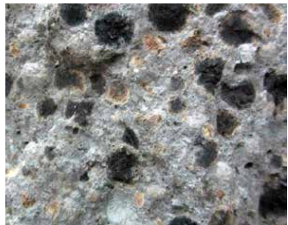
A View of Concrete made with Light Weight Coarse Aggregate
