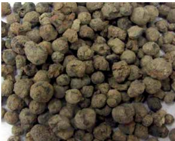
Sintered Fly Ash based Light Weight Coarse Aggregate
