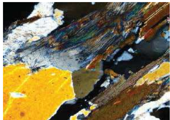
Core-II-2: Distribution of quartz, biotite, orthoclase-feldspar, muscovite and iron oxide grains in the rock (5x, x-nicols)
