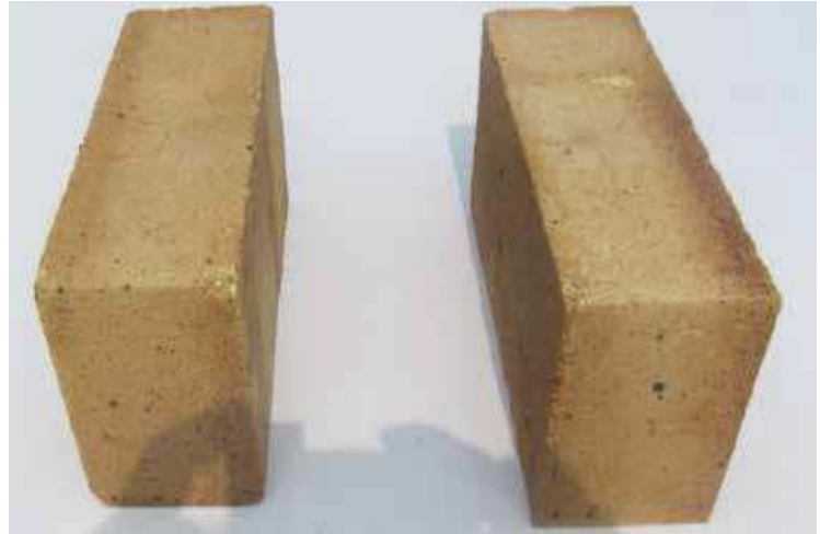
Photograph showing the fired Refractory Bricks manufactured using Alumina Waste
