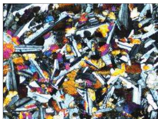
Optical Micrograph of Basalt Sample showing distribution of different mineral phases
