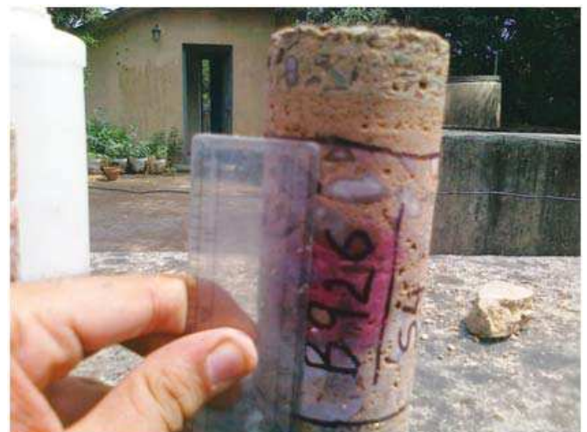
Core extracted from terrace of a Residential Township showing carbonation depth
