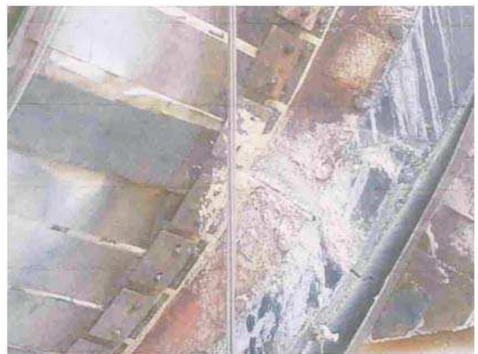
View of deformed outlet air seals as observed during the technical (health) audit
