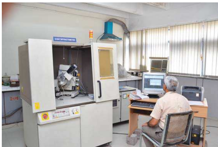
X-ray Diffractometer (XRD) for Mineralogical Analysis of clinker and raw materials of cement
