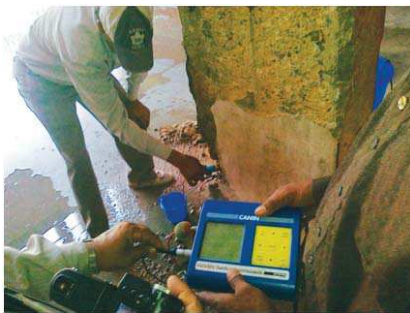
Half-cell potential test being done on a column
